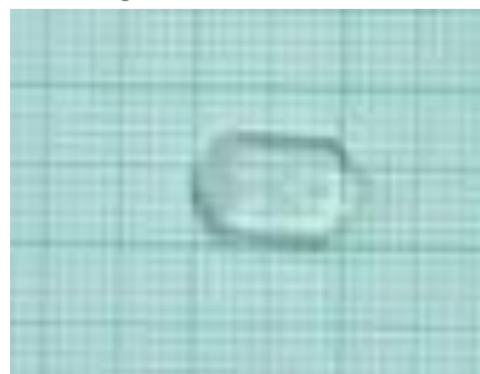
Fig.3 Silver nitrate doped KDP
